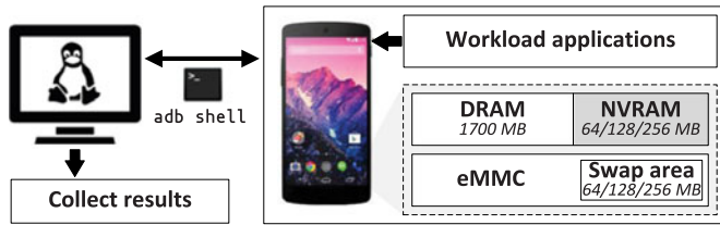
Fig. 5. The experimental setup. We conduct the experiments on Google Nexus 5 and use adb tool to communicate with it.
